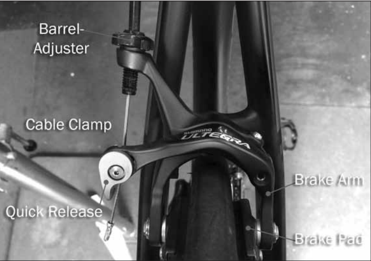
Caliper brakes are found on most road bikes. Photos courtesy of Cycle U
