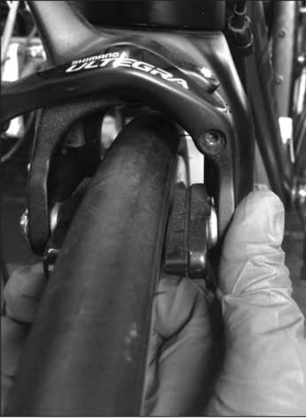
Aligning the brake pads.
