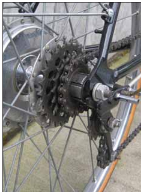
d. Trivelox shifters moved the cogs and kept the derailleur in a fixed position.
