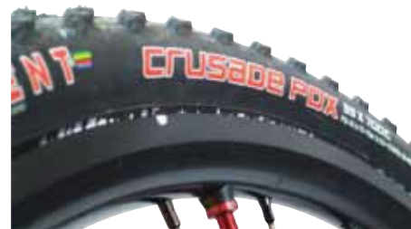
Tubeless tire sealant bubbles around the edge sealing the air in.
