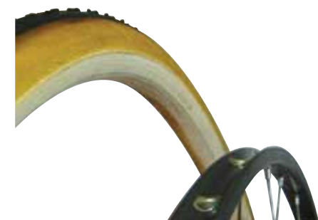
Tubular (sew-up) tire and a tubular rim.
