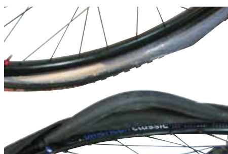
Same tire set up tubeless (top) and with inner tube (bottom).
