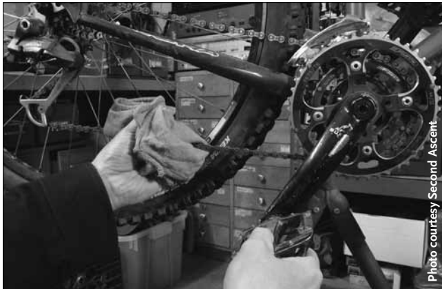
To clean, pedal backwards and let the chain run through the rag.
