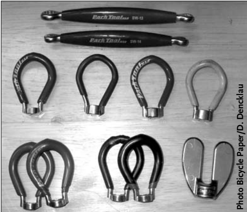
With so many different sizes of spoke wrenches, it is important to choose the right one.
