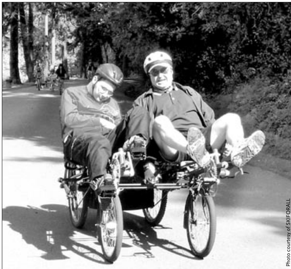
Ryland McGill and SKIFORALL volunteer Dennis Flynn pedal a JustTwo Bikes/JTB side-by-side tandem cycle. Independently geared (21 speeds). Both cyclists can pedal and brake, but only one can steer.
