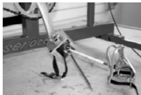
RAD-Fits, a part of a Fit Kit, is used for foot/pedal interface.
