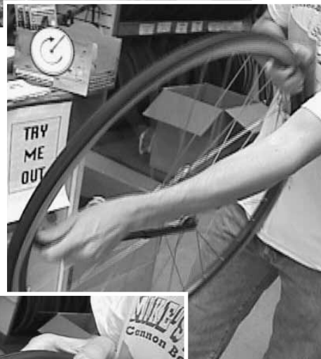
Step Three Rotate to lever the bead from the rim. Even the toughest tires are a breeze to re- move.
