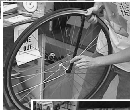
Step Two Telescope down to use the axle as a pivot.
