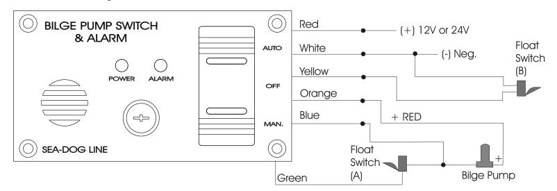
Use min. #16 gauge marine grade electrical wire.
