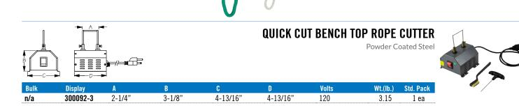
This Quick Cut Bench Top Rope Cutter easily cuts and heat seals nylon, polyester, polypropylene, and Dacron cordage and webbing. The replaceable blade heats up to 1000° Fahrenheit (500° Celsius) in 10 seconds. Includes brass bristle cleaning brush and T-handle Allen wrench for installing the replaceable blade. Features a 39" heavy duty grounded cord and a lighted on/off rocker switch. Base is pre-drilled for permanent mounting on a bench or table. 120VAC @ 30W. ETL certified #5002516.
