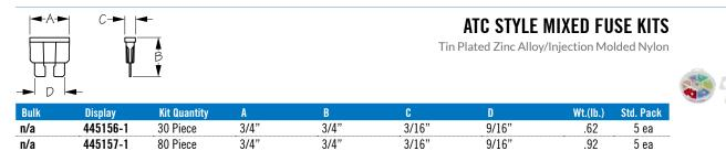
ATC Style Mixed Fuse Kits contain fast acting ATC (closed) fuses to provide better protection for electronic devices. 30 piece includes five 3A, five 5A, five 10A, five 15A, five 20A, and five 30A. The 80 piece includes fifteen 3A, fifteen 5A, fifteen 10A, fifteen 15A, ten 20A, and ten 30A. Constructed of injection molded nylon with tin plated connector blades for superior conductivity and improved corrosion resistance.
