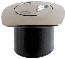
The LED Pop-Out Combination Bow Light is approved for USCG 2 NM (Colreg 2 mile). A simple twist of the cap allows the light to pop up, ready to use when it's switched on. Push the cap down, twist to lock, and light disappears into the deck. Constructed of corrosion resistant investment cast stainless steel cap and bezel. Installs with three #10 fasteners (included). IP67 waterproof rating.
