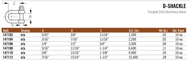
D-Shackles have straight sides with a U-shape bottom. The U-shaped end can handle heavy loads even on the straight sides (may cause bending). Designed for rigging with bi-directional loads. Constructed of corrosion resistant forged 316 stainless steel.
