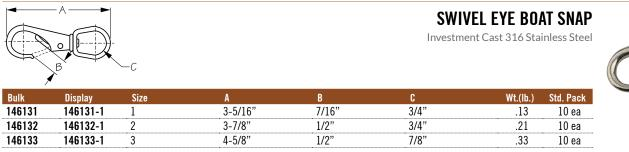
These Swivel Eye Boat Snaps feature a spring-loaded latch for easy attachment. Designed for medium duty rigging applications. 360° swivel eye eliminates tangling. Constructed of corrosion resistant investment cast 316 stainless steel. Also see die cast zinc chrome plated Swivel Eye Boat Snap (148131).
