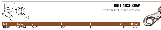
This Bull Nose Snap features a spring-loaded latch for easy attachment. Designed for medium duty rigging applications. 360° swivel eye eliminates tangling. Constructed of corrosion resistant investment cast 316 stainless steel. Also see cast zinc chrome plated Bull Nose Snap (148333).
